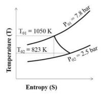
Assuming specific heat ratio of 1.33 for the hot gas, the isentropic efficiency of the turbine stage is \_\_\_\_\_\_\_%(round off to two decimal places).
